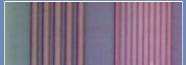
1um and 500 nm lines patterned using resistless and solventless lithography from joint SRC/NSF ERC in Environmentally Benign Semiconductor Manufacturing.
