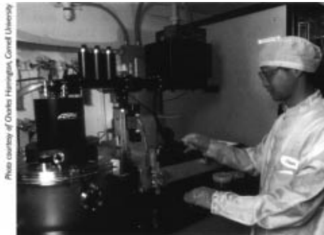
Ph.D. student S. Chieh fabricates 0.1 μm MOS transistors in the Cornell University Nanofabrication Facility.
