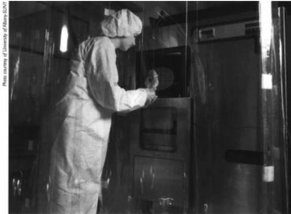
The SRC Research Catalog helps industry track and assess SRC-sponsored university research, such as this work in advanced thin film technology at the University of Albany-SUNY. Here, Albany's Cindy Goldberg loads an 8" wafer for CVD thin film deposition.
