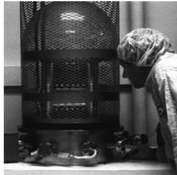
Cornell student Martin Van Derhiede operates a controlled atmosphere reflow unit to prepare a solder joint specimen for fatigue testing.
