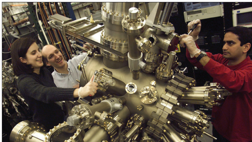
From l-r: Lisa Edge, Darrel Schlom, and Venugopalan Vaithyanathan with an oxide molecular-beam epitaxy (MBE) system, in which high-k alternative gate dielectric materials are grown on silicon. Photo by Cramer Studio.
