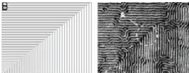
Figure 3. (a) Epitaxial assembly of block copolymers in 'L' patterns on (b) chemically nanopatterned substrates. (Nealey, Kim, Solak; Univ. of Wisconsin-Madison; unpublished results.)
