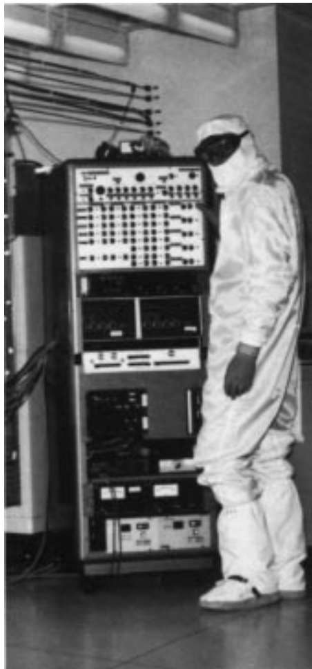
SRC Fellow James Comfort with plasma-enhanced epitaxial silicon reactor in the new clean room at MIT. (See "Low-Temperature Epitaxy" research highlight on page 12.)
