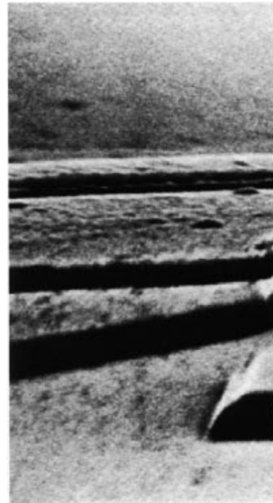
Fully self-aligned, surface channel quarter-micron NMOS device.
